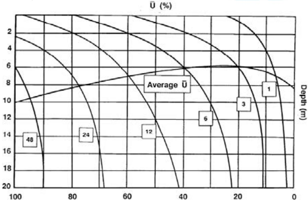
Fig. 7 –Effect of drain depth on consolidation time
