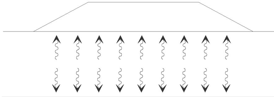
Fig. 4 – Consolidation without prefabricated vertical drains
