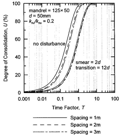
Fig. 7. Effect of PVD spacing on consolidation rate
