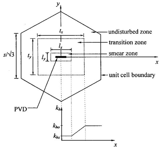
Fig. 1. Hexagonal unit cell with rectangular disturbed zone
