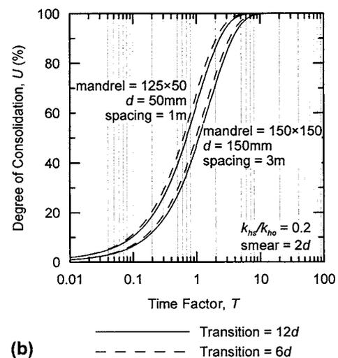
Fig. 4. Effect of disturbed zone dimension on consolidation rate: (a) effect of smear zone dimension; (b) effect of transition zone dimension
