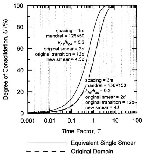
**Fig. 9.** Replacement of original domain with smear and transition zones by an equivalent domain with an expanded smear zone
