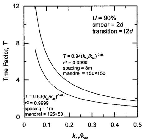
Fig. 6. Dependence of time factor on the degree of disturbance
