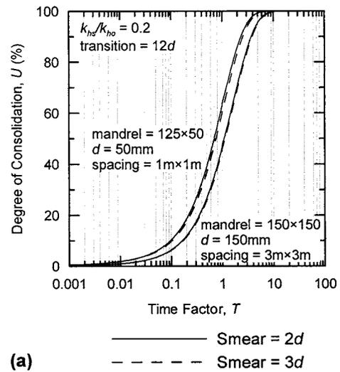
Fig. 3. Effect of soil disturbance on consolidation rate
