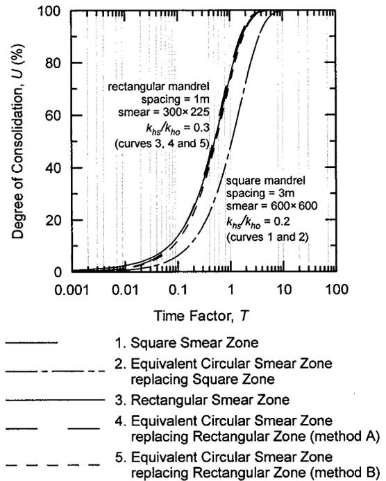
**Fig. 10.**  $U$  versus  $T$  curves for square, rectangular, and equivalent circular smear zones (Curves 1 and 2 are almost coincident; Curves 3–5 are very close to each other, with Curve 3 lying to the right of Curve 4 and to the left of Curve 5 for  $T > 0.5$ )
