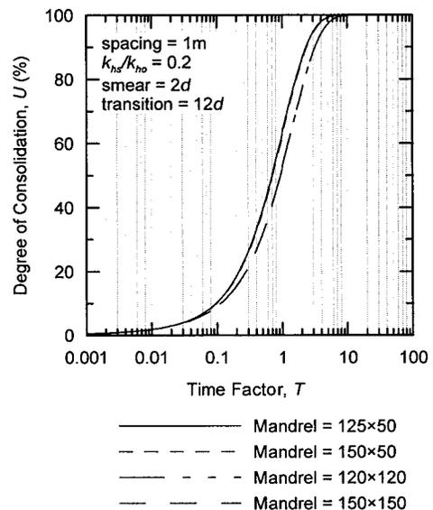
Fig. 8. Effect of mandrel size on consolidation rate (the curves for the  $125 \times 25$  mm mandrel and the  $125 \times 50$  mm mandrel almost coincide; this is also the case for the curves of the  $120 \times 120$  mm mandrel and the  $150 \times 150$  mm mandrel)
