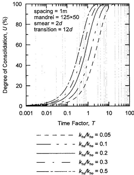
Fig. 5. Effect of degree of disturbance on consolidation rate
