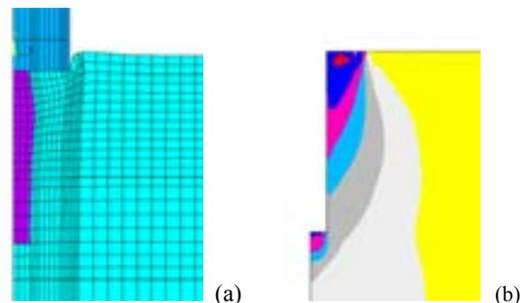
Fig. 1. Deformed mesh (a) and vertical stresses in the soil (b)
