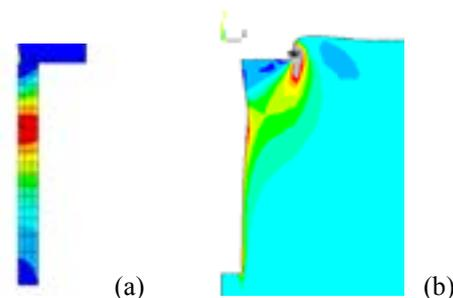
Fig. 2. Plastic deformation in the column (a) and the surrounding soil (b) during bulging
