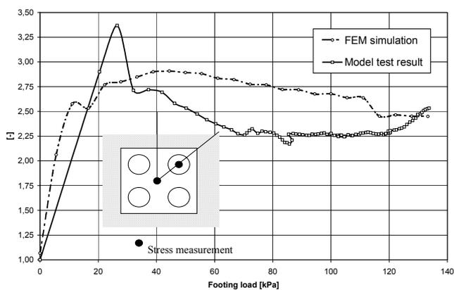
Fig. 8. Ratio of the vertical stresses on column and soil over footing pressure
