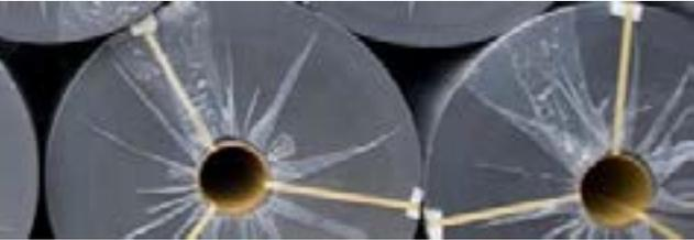
They have the ability to separate, filter, reinforce, protect, or drain. Base material is polypropylene or polyester, geotextile fabrics come in three basic forms: woven, needle punched, or heat bonded.
